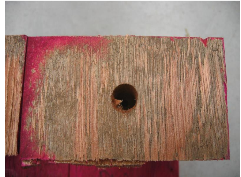
PVAC glue (D4 type) on meranti after 6 wks artificial weathering and stain test
